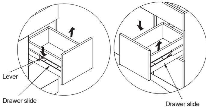
**Step 1:** Release the lever on each drawer slide (push the lever on the left drawer slide downward and the lever on the right drawer slide upward) to release the drawer from the cabinet. **NOTE:** to remove the drawer, hold the lever in place and firmly pull the drawer out.
