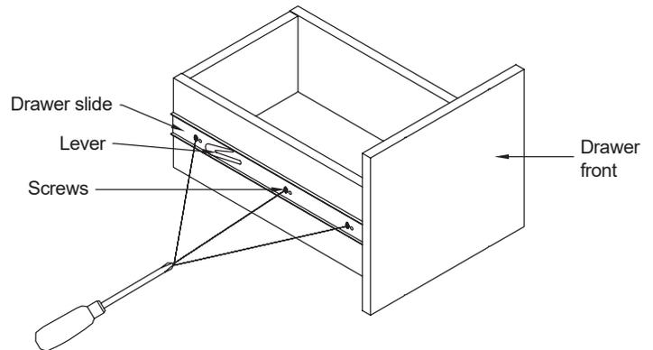
**Step 2:** Using a Phillips screwdriver, loosen the screws that fasten the drawer slide to the drawer. Shift the drawer slide as needed (up or down / in or out). Re-tighten the screws and repeat for the opposite side as necessary. To place the drawer back into the cabinet, align the drawer slides with the cabinet slides and push firmly until the drawer is secured into place.
